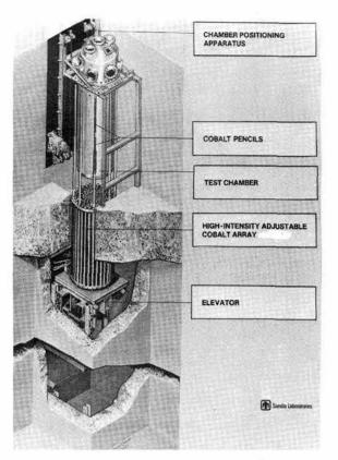
NEW Labs facility can simultaneously subject reactor safety equipment to multiple environments—high temperature, pressure, chemical and radiation. Conditions simulate those anticipated in a loss of coolant or steam line break accident.
